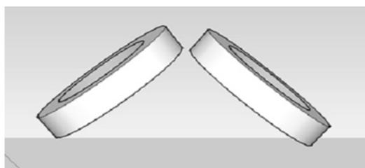
Fig. 6. Inverted V coil
